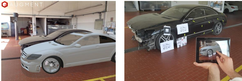
Figure 3 – Visual presentation of vehicles in the process of crash forensics using Augmented Reality.
