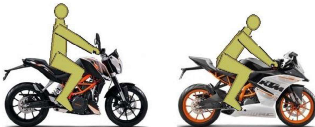
Fig. 3. The rider's position in a street style motorcycle (on the left) and in a sport style motorcycle (on the right)
