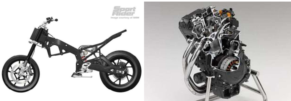
Fig. 2. Chassis of BMWXR 1000 (a); Parallel twin engine of Honda 500cc (b)
