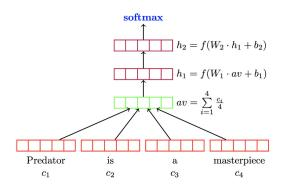
FIGURE 3. USE based on DAN architecture [2].
