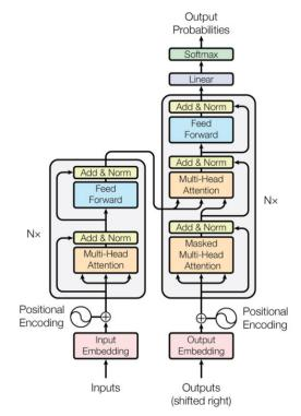
FIGURE 5. The Transformer architecture [59].
