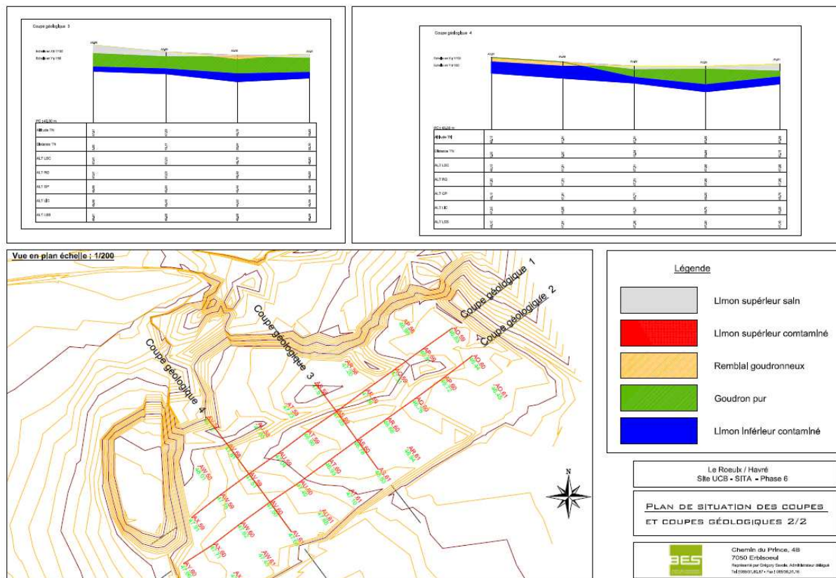
Fig. 2. Map with geological sections of the acid tar area. In green, the acid tar layer. In blue, the silt layer.
