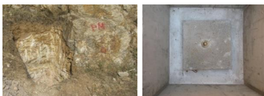
Figure 9. Stabilization of the fundamental benchmark
