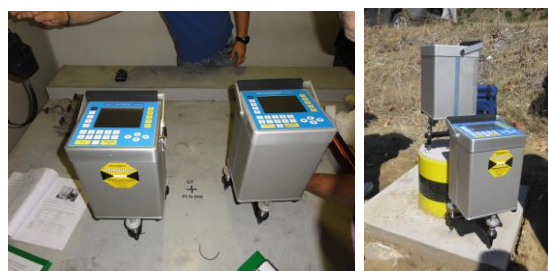
Figure 3. a) Stationing at absolute gravimetric point; b) stationing at points from First Order Gravity Network
