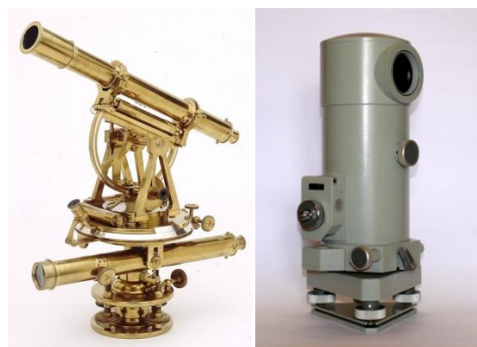
Figure 6. Classical geodetic instruments: Brass theodolite and Koni 007 leveling instrument
