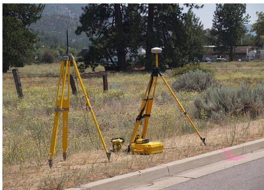
Figure 8. Modern GNSS instrument Trimble R6
