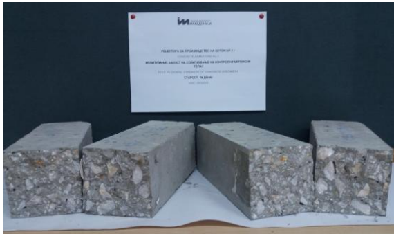
Figure 11. Tested specimens for flexural strength
