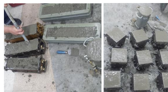
Figure 2. Preparing of concrete samples
