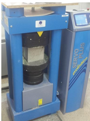
Figure 3. Press for testing compressive strength
