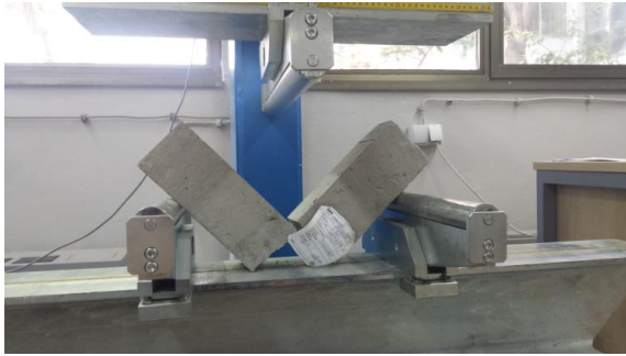
Figure 10. Prisms tested to bending
