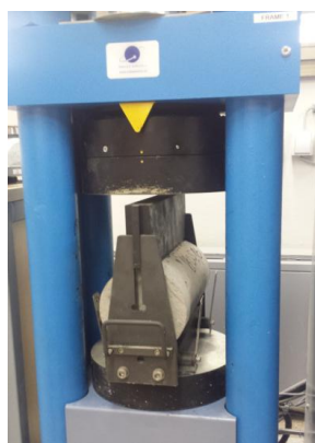
Figure 7. Brazilian method - testing of specimen with splitting test
