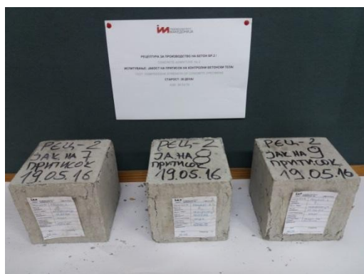
Figure 4. Tested cubes of recipe 2 for compressive strength at 28 days
