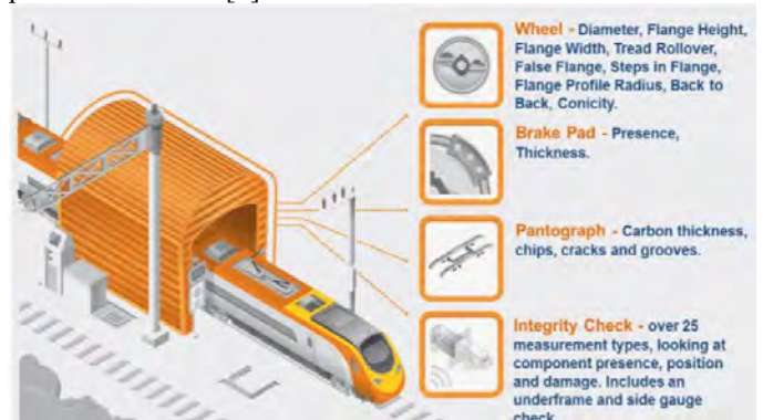
Fig. 6 “HealthHub” wayside monitoring system [9]
