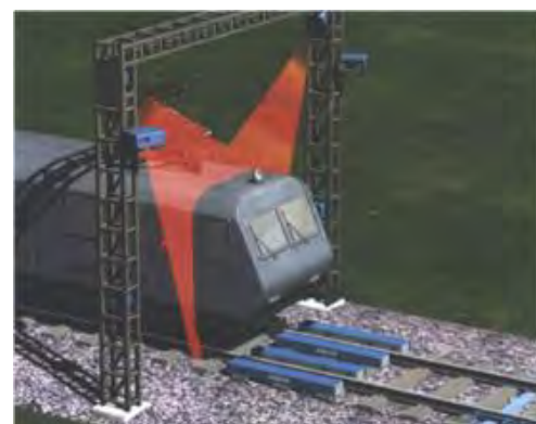
Fig. 2 System for train gauge control
