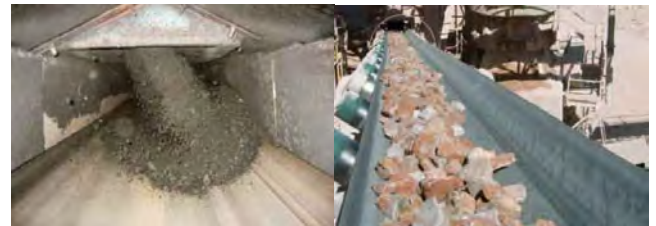
Fig. 6 Off-center feeding of the material on the belt (left) and belt misalignment (right)
