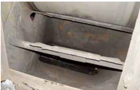
Fig. 14 Deflector placed in the upper part of the feeding hopper
