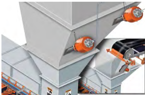
Fig. 9 Air cannons installed on the feeding hopper
