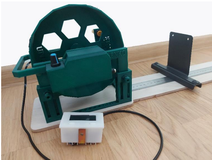
Figure 1 – Equipment for measuring the throughput of RFID readers
