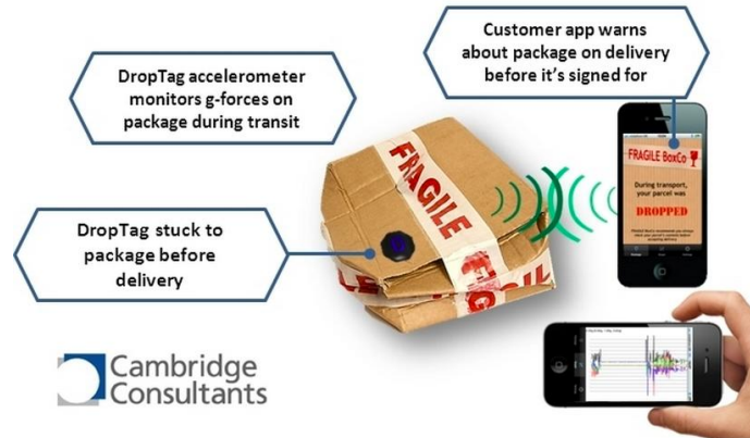
Figure 2. DropTag allows the identification of product damages [Cambridge Consultants, 2013].
