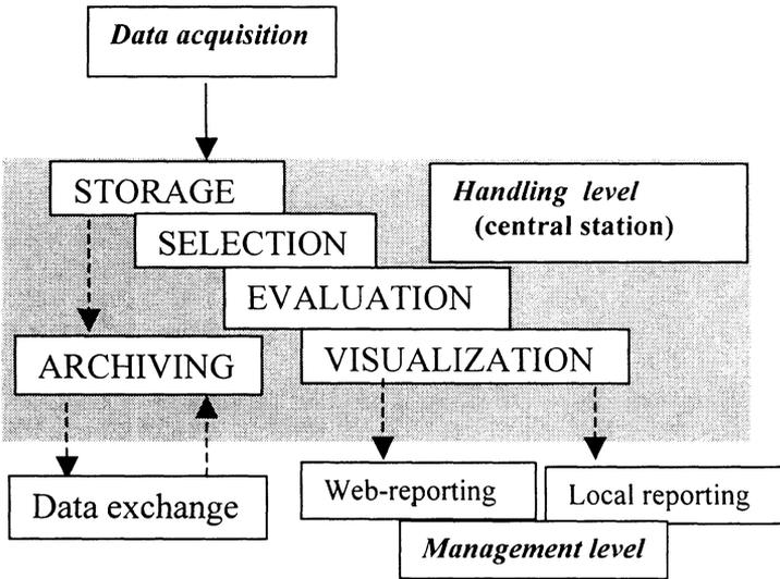
Fig.1 Process steps of monitoring system
