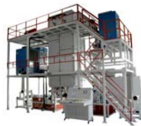
Fig. 4. Vertical impregnating machine LI 300
