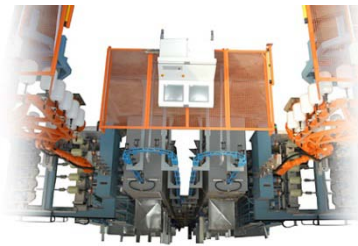
Fig. 6. Automated FW machine (Source: Mikrosam [9])
