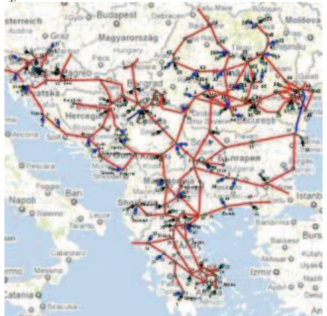
Figure 1. Electric power grid of Southeast Europe
