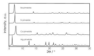
Fig. 4. Scattered X-ray intensities of the synthesized pimelates
