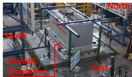
Fig. 16. The test for the scaled model of superstructure and periodic foundations.
