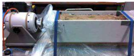
Figure 17 – Experimental setup for array of resonators
