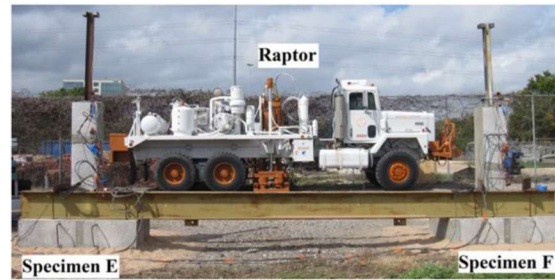
Figure 20 – Experimental setup for 1D metamaterial foundation
