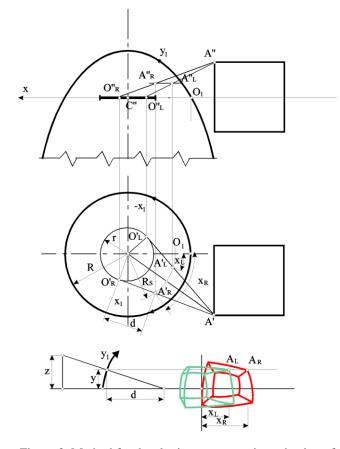
Figure 3. Method for developing stereometric projection of a cube in a paraboloid projective space
