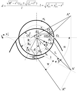
Figure 4. Graphical representation of the mathematical model for stereometric projection in a paraboloid projective space
