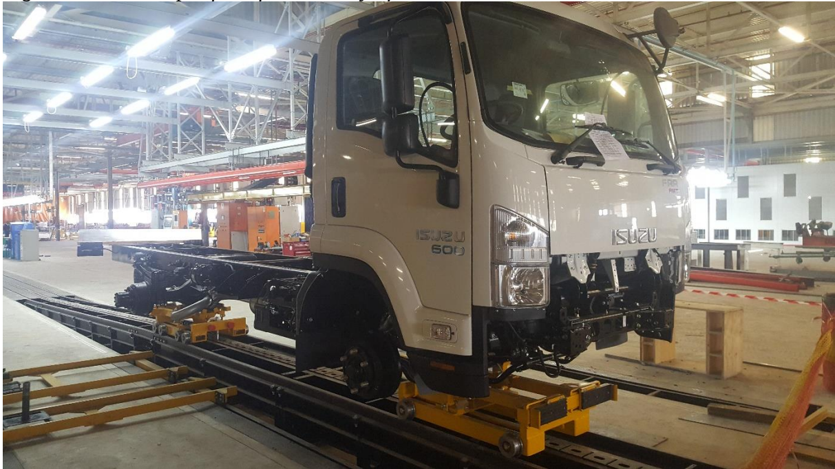
Figure 5: Foldable platform for assembly of trucks
