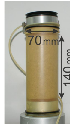
Fig. 9. Soil specimen on a triaxial apparatus.
