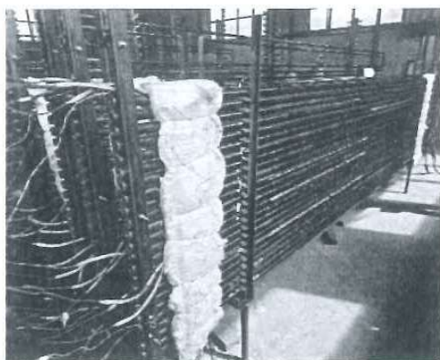
Figure 1. PWHT of X10CrMoVNb9-1 and 10CrMo9-10
