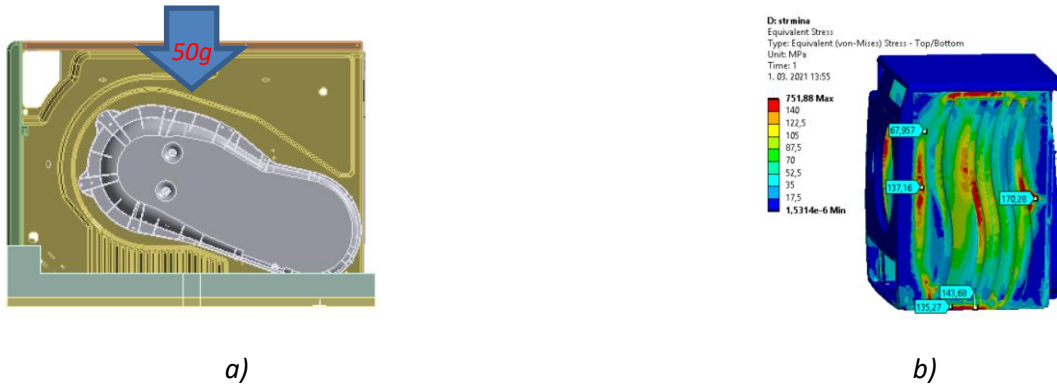
Figure 6: The simulation of impact on the sidewall during slope test; a) Application of acceleration loads, b) Stresses on the appliance during impact.
