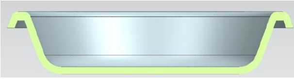
Figure 4: Cross-section of the crucible model
