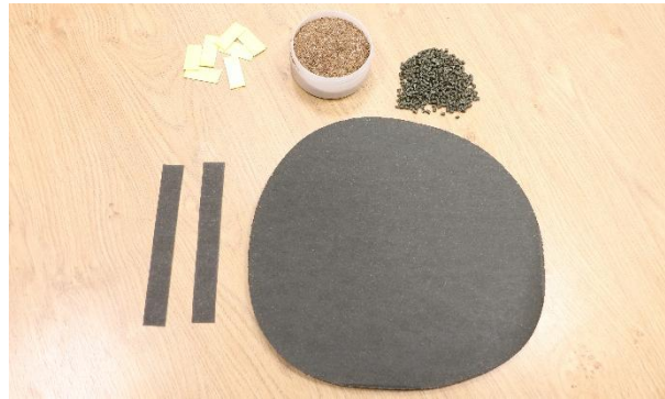
Figure 1: PP packing belts (top left), waste coconut fiber (top middle), biocomposite granulate with 20 wt.% waste coconut fiber (top right), samples cut from the sheet used for laboratory tests (bottom left) and composite sheet (bottom right)
