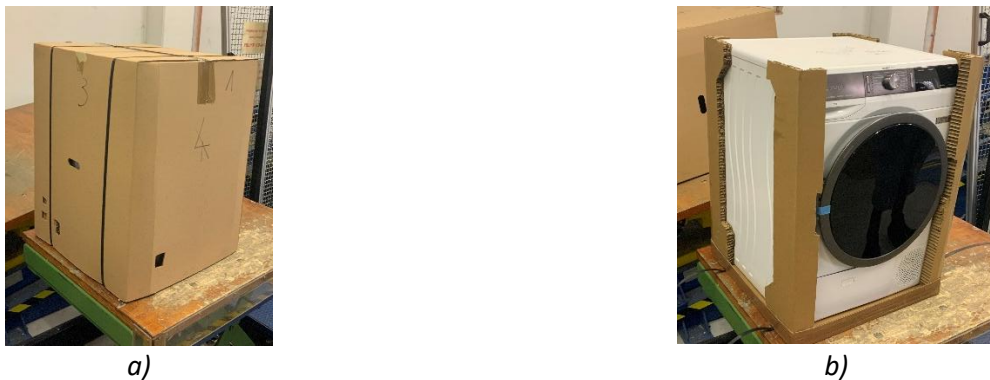
Figure 7: The actual prototype of paper honeycomb packaging; a) Packaged appliance in cardboard box, b) Inner view of packaging design.
