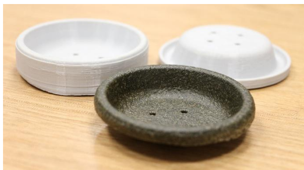
Figure 8: Male version of the tool (top right), female version of the tool (top left), and pot for growing plants with hydroponics (bottom middle)
