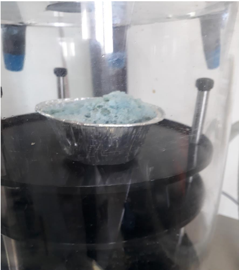
Fig.2: Enriched with %5 Spirulina solution sample's foam problem in freeze dryer
