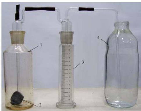
Figure 1. Equipment for determination of the rate of steel wool rusting. 1 – reaction chamber; 2 – steel wool; 3 – graduated glass cylinder; 4 – reservoir of water.
