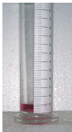
Figure 2. The so-called 'zero volume', 45 minutes after the experiment begun. All measurements are referred with respect to it.
