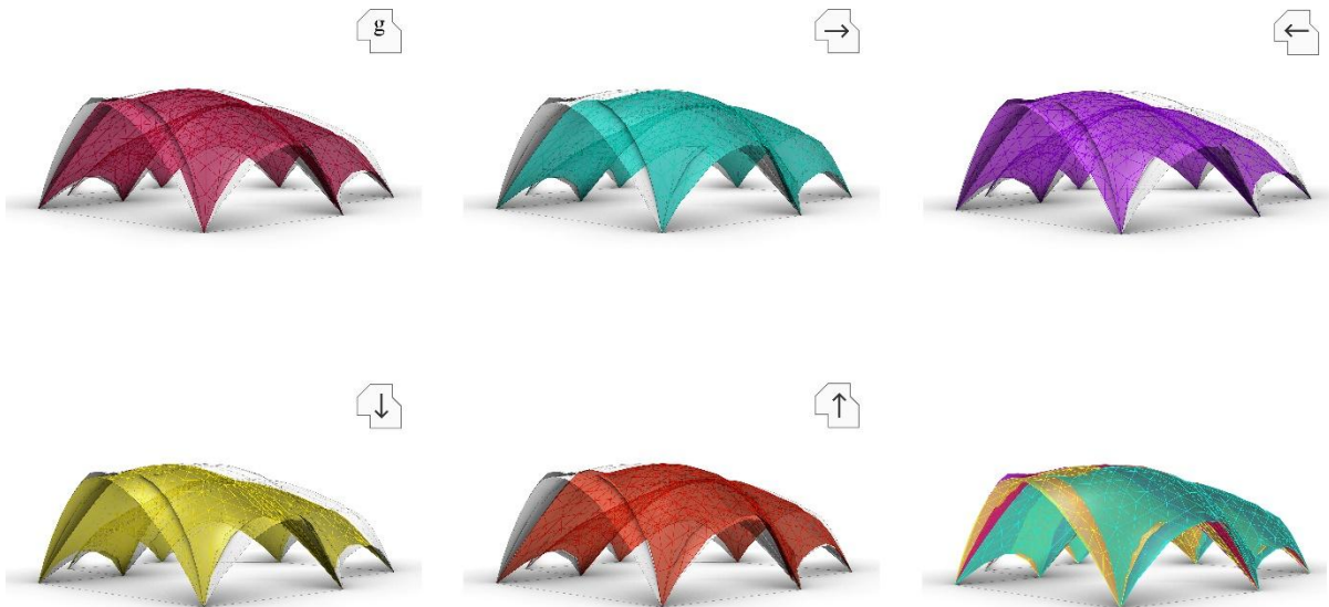
Figure 2– Superimposed funicular nets that are obtained through dynamic relaxation for earthquake loading in different directions.
