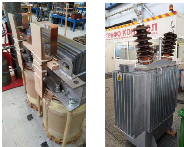
Fig. 5. Manufactured Booster Transformer (200 Amps) subject to research
