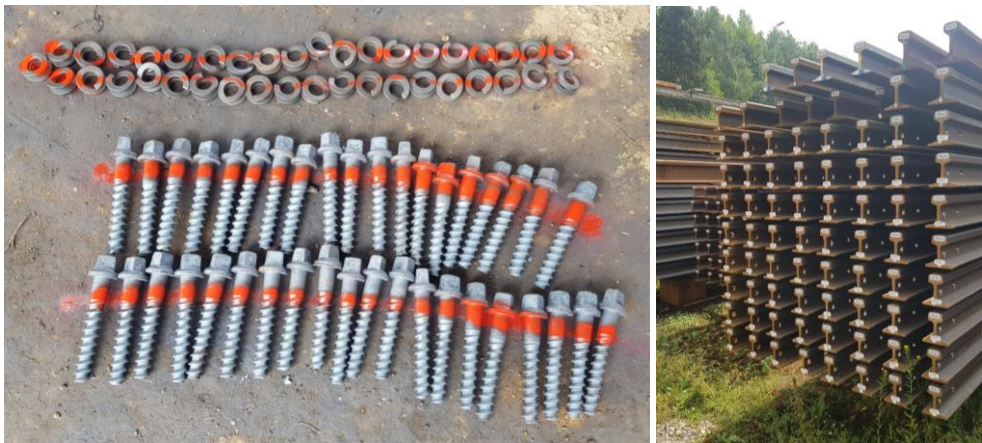
Figure 2. a) Taking Over of fastenings for testing; b) Taking Over of rails 49 E1 R350HT, Leoben, Austria
