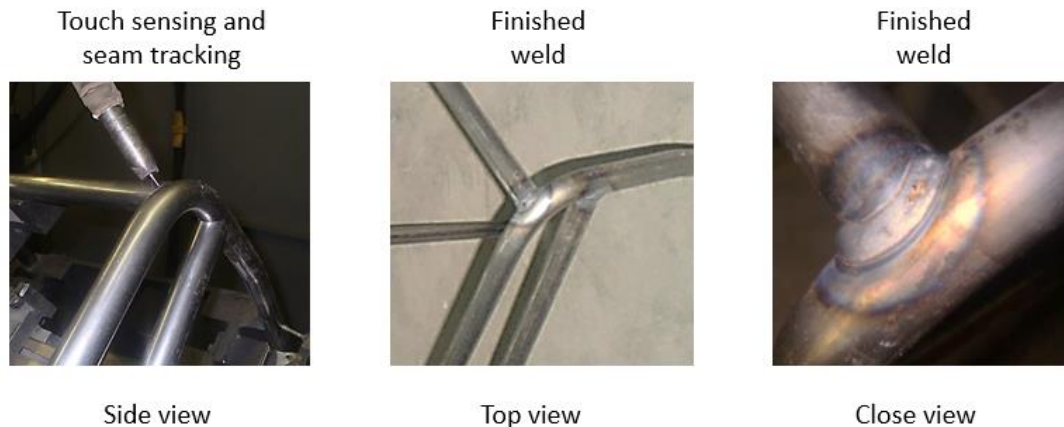
Fig. 6. Touch sensing and finished weld
