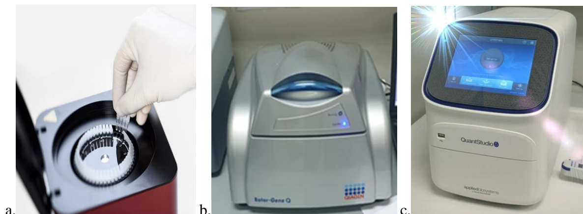
Figure 21. a. MIC 4 real-time PCR thermocycler Bio Molecular System (Upper Coomera, Australia); b. Rotorgen Q real-time PCR thermocycler QIAGEN (Hilden, Germany); c. QuantStudio 5 real-time PCR thermocycler Thermo Fisher Scientific, (Waltham, USA).
