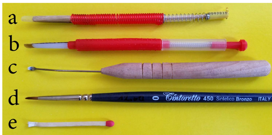
Figure 5. Grafting tools: (a) “Chinese”; (b) modern version of “Chinese”; (c) metal grafting spoon; (d) fine brush; (e) flattened match. Photo: J Wilde.
