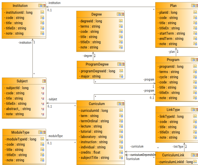
Fig. 3. Class diagram of the structure of study plans in each institution, with study programs and offered degrees, curricula per program for each subject domain, and graph structure showing the full graph of links between curricula allowing many types of links.
