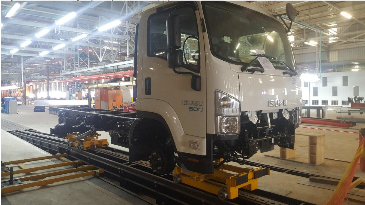
Figure 5: Foldable platform for assembly of trucks
