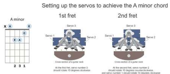
Fig. 7. Example of servo positions on first three frets for A Minor chord
