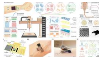
Fig. 4. 3D-printed e-skin is composed of an array of electrochemical sweat biosensors(glucose, alcohol, and pH sensors) and biophysical sensors (temperature and pulse sensors)
