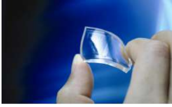
Fig. 3. Stretchable graphene electrode patterns transferred onto a silicon based polymer
