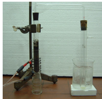
Fig. 3. Synthesis of acrolein – end of reaction (the black color is due to part of the glycerol being oxidized to carbon)
