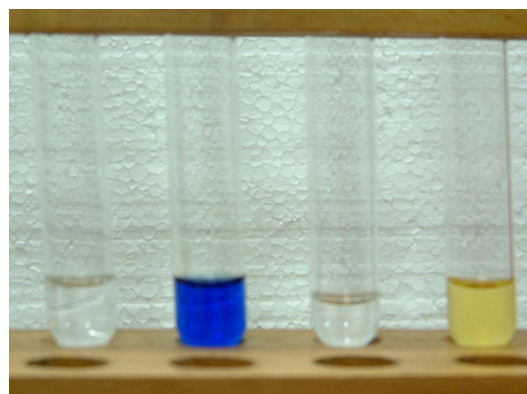
Fig. 2. Test-tubes in the rack are filled with (left to right): Nylander, Fehling, Tollens reagent and (the rightmost one) bromine water
