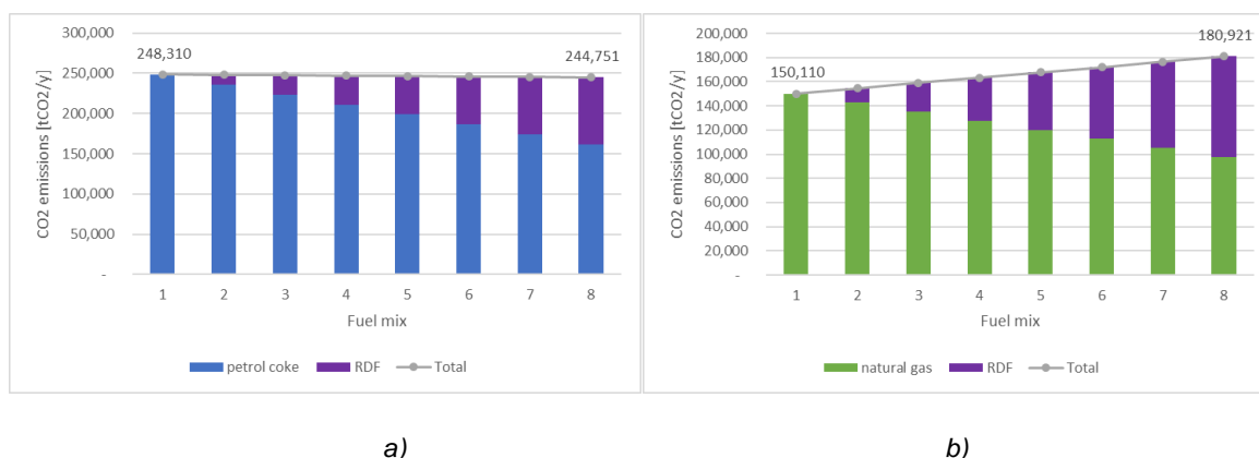
Figure 6: CO 2 emissions trend from combustion RDF with a) petrol coke, b) natural gas
