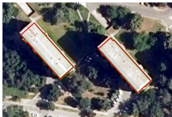
Figure 3. Buildings registered in the cadastral system (green polygon), detected buildings based on LiDAR data (red polygon)
