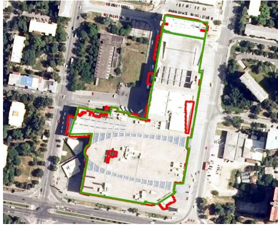
Figure 7. Building registered in the cadastral system (green polygon), detected building based on LiDAR data (red polygon) – Skopje City Mall
