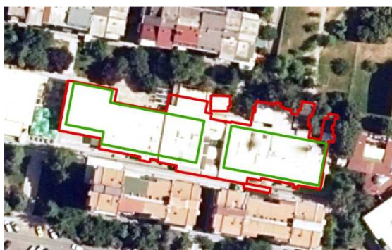
Figure 14. Buildings registered in the cadastral system (green polygon), detected building footprint based on LiDAR data (red polygon)
