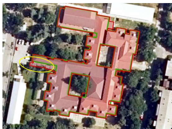
Figure 5. Building registered in the cadastral system (green polygon), detected building based on LiDAR data (red polygon)
