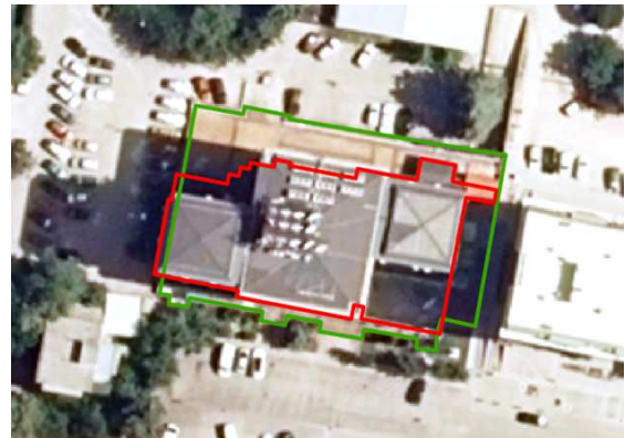
Figure 10. Building registered in the cadastral system (green polygon), detected building footprint based on LiDAR data (red polygon)
