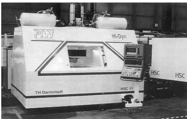
Fig. 5 High Speed Cutting CNC linear motor machine (HSC 11) at the Institute of Production Management, Technology and Machine Tools (PTW) at Technical University Darmstadt, Germany
