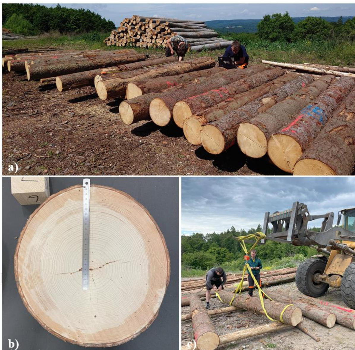
Figure 1. Measuring area at the Sawmill Olomučany (a); Sample for the determination of the moisture content (b); Weighing of logs (c).
