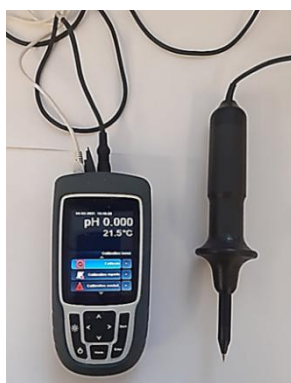
Figure 3. SENTRON pH meter SI 600 series with LanceFET+H probe 22704-010.
