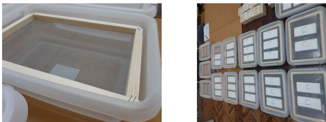
Figure 3. Testing the water-vapour permeability: a) containers filled with water with grid frame on top and b) samples placed faced to water by wide side
