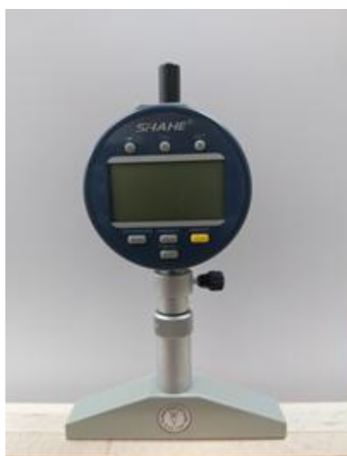
Figure 2. Digital comparator type SHAHE.
