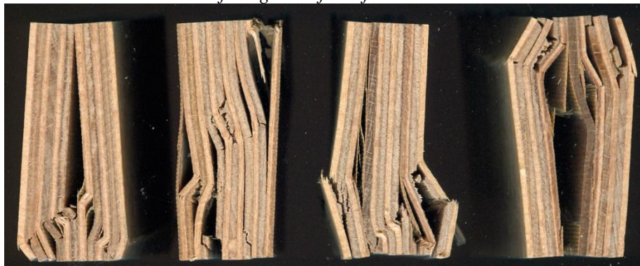
Figure 8. Failure mode of the test specimens of reinforced models during testing the compressive strength parallel to the face grain.
