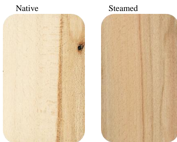
Figure 1. Wood color of unsteamed beech wood with false heartwood (native) and steamed.
