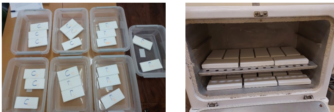
Figure 2. Preconditioning of the samples: a) immersing of the samples in water for 24 hours and b) drying of the samples at a temperature of 50 °C for 3 hours.
