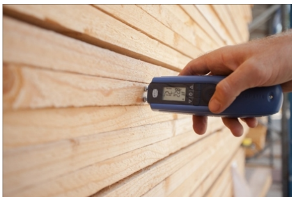
Figure 2. Measuring moisture content in wood.
