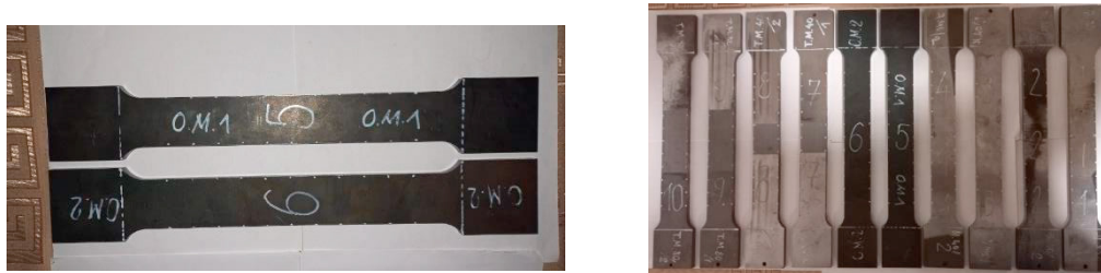
Fig.6: Preparation of samples by addition of liquid super metal, Belzona
