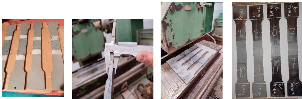
Fig.6: Preparation of samples by addition of liquid super metal, Belzona
