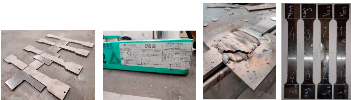
Fig.5: Preparation of samples by repair welding
