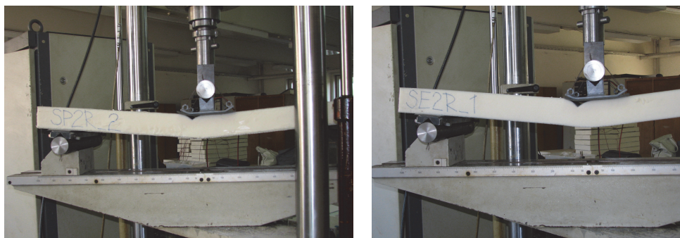
Figure 5. Fracture of the sandwich panels SP2R and SE2R subjected on three points bending
