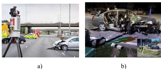
Fig. 6 Laser Scanning of a crash site. a) Scanning an accident site, b) Measuring important distances using CAD software based on the data acquired by laser scanning. (Source: MAPTEK; 2016).
