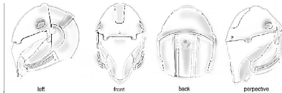
Figure. 11: Side, front, back and perspective view of the second concept design.
