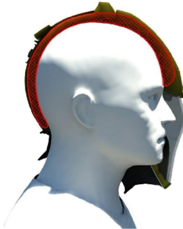
Figure. 17: Head inlay with polyurethane.
