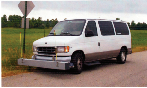
Fig. 2. The Dynatest Road Surface Profilometer ® 5.051 Mark II
