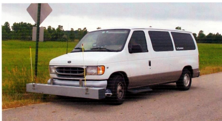
Fig. 4: Inertial profilometer type: The Dynatest Road Surface Profilometer 5.051 Mark II
