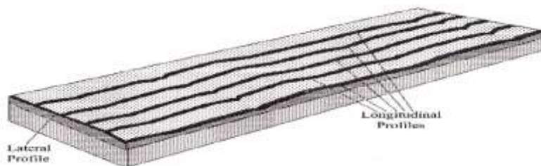
Figure 2. Types of unevenness of pavement surface Source: (Sayers, M.W.; Karamihas, S.M., 1998. The Little Book of Profiling)
