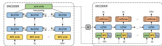
FIGURE 4. LASER architecture [33].
