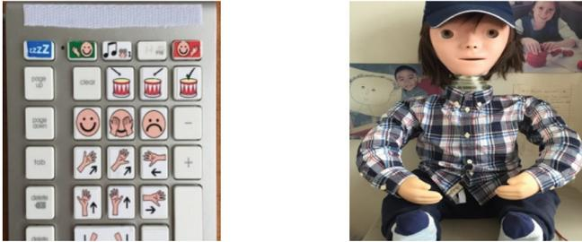
**Fig. 1.** Wireless keypad for manual control (left); The Kaspar robot (right)
