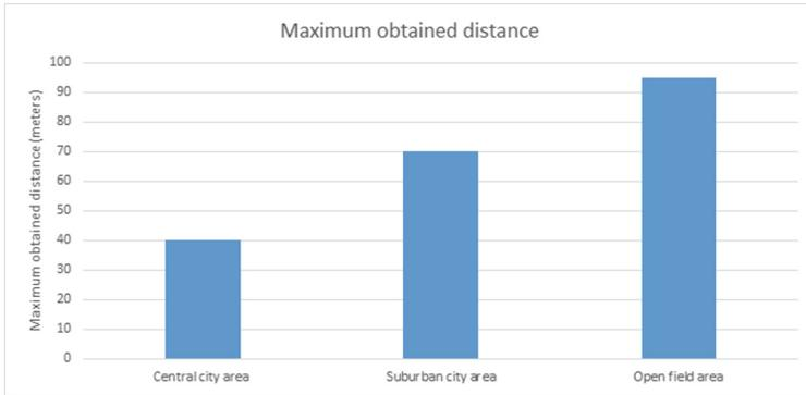
**Fig. 12.** Maximum obtained distance in various environments
