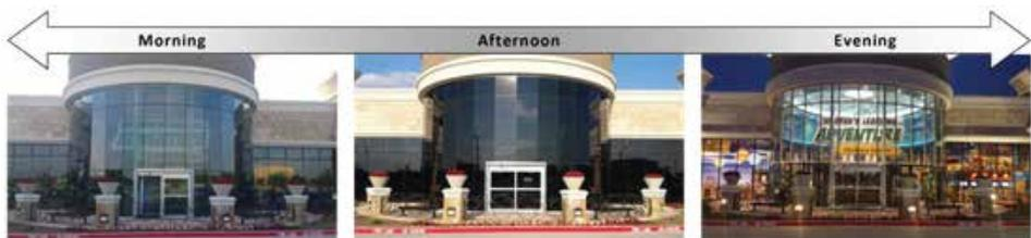
**Fig. 1.** Suntuitive glass windows (thermotropic glass) installed at an educational facility in Keller, Texas, USA
