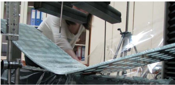
Fig. 4. Full hybrid element failure
