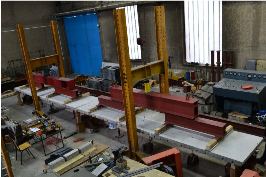
Figure 11. Composite beam subjected to the testing
