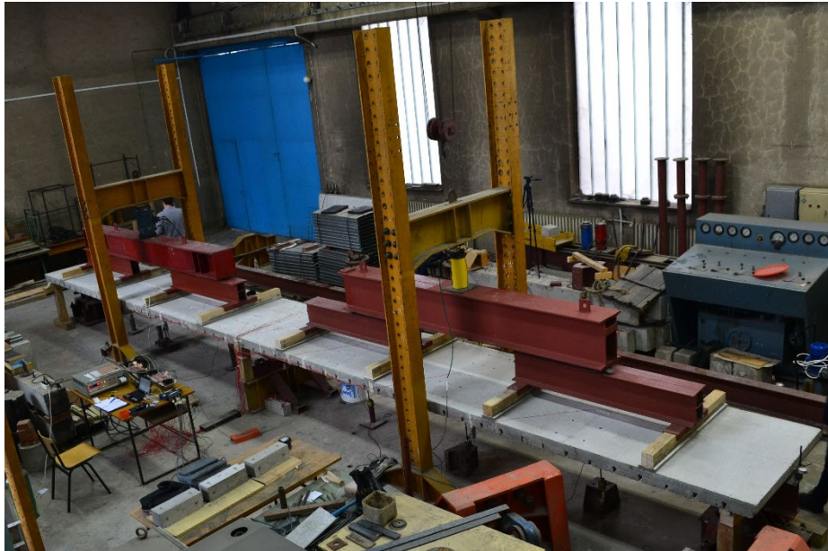
Figure 5. Composite beam subjected to the testing
