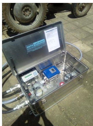
Figure 2. Pumptester and flowmeter- AAMS-SALVARANI
