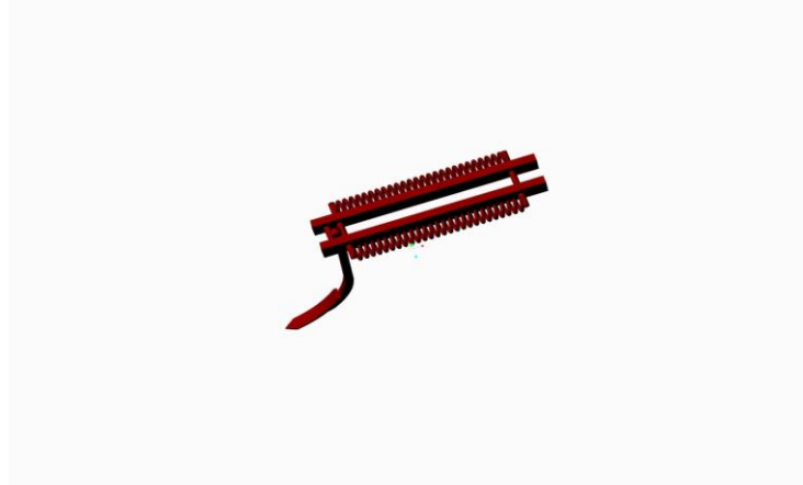
Fig. 7 Spring loaded Reversible tine used in the Developed Machine
