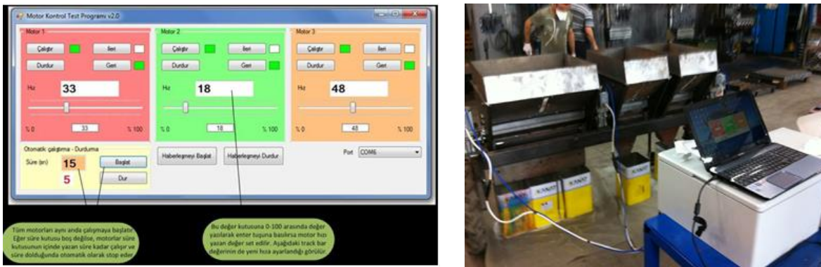
Figure 5. Laboratory test software for variable rate controllers
