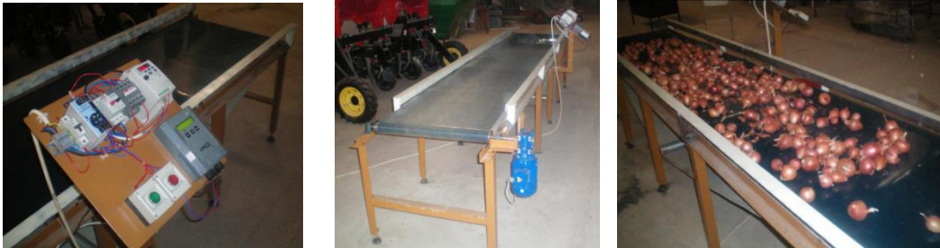
Figure 7. Weight measurement system of conveyor for tuber crops
